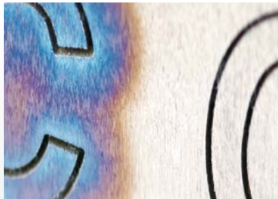
Surface machined with a conventional generator: deposits and pollution Surface machined with the CC: minimal deposits, smooth surface
