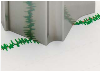
H40S CF Carbide Ra 0.10 \mu\text{m} Rt 0.88 \mu\text{m} Rz 0.71 \mu\text{m}
