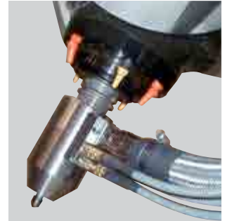
Motor-driven spindle for 60,000 rpm
