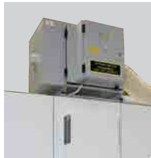
Suction removal of mist
