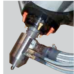
Motor-driven spindle for 60,000 rpm
