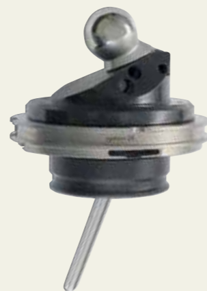
Matrix application: Pallet with special fixture for protruding workpiece in this case a "hip joint"
