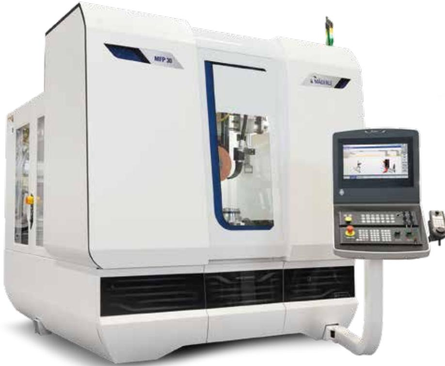
The compact MFP 30 5-axis grinding center from MÄGERLE is ideally suited for grinding complex geometries, particularly those of blades and vanes or heat shields for aviation turbines. The workpieces to be machined are ergonomically loaded into the work area directly from the front. Heavy workpieces with a clamping fixture can be loaded from the top using a crane. The compact and space-saving design allows optimal use of the available production area and enables an effective production flow.
