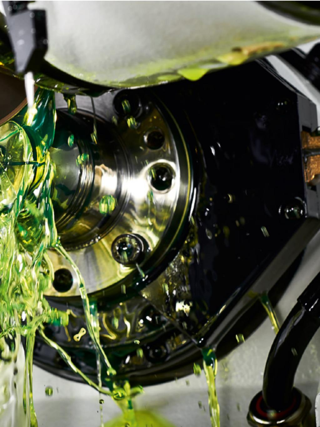
With FINE PULSE TECHNOLOGY, the HELITRONIC VISION DIAMOND 400 L sets new benchmarks for quality for PCD tools. It is an economic investment for both the production and sharpening of PCD/CBN tools in the diameter range of up to 315 mm.
