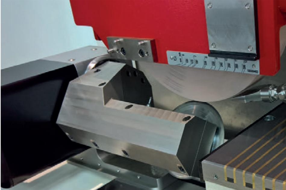
**Swivel dresser** PA-T130 mounted on the left of the machine table. Torsion-resistant dressing arm mounted on one side for a  $\mu\text{m}$ -accurate contour and fast tool change. Automatic adjustment of the dressing wheels (profile depth up to 30 mm).
