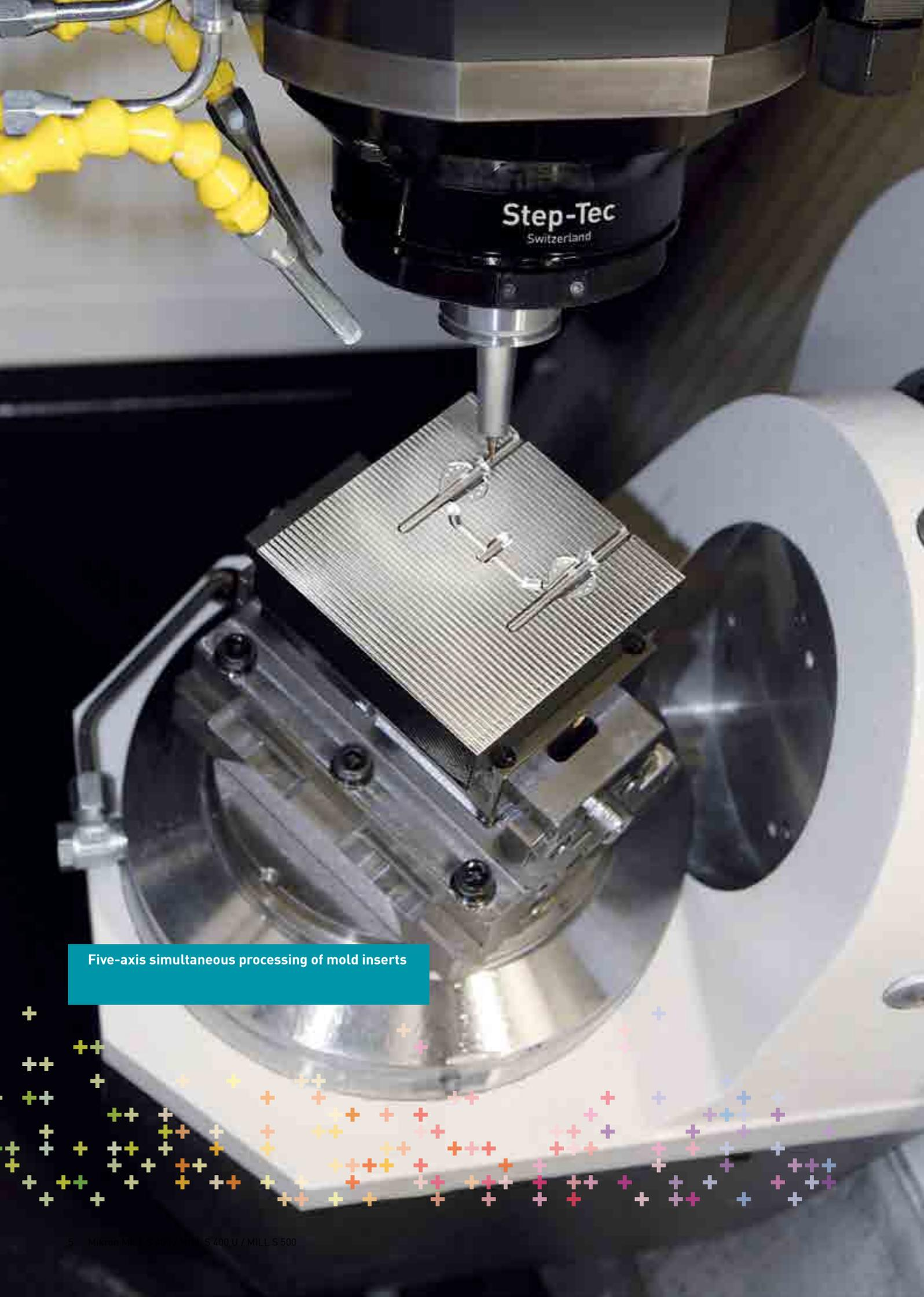
Five-axis simultaneous processing of mold inserts
