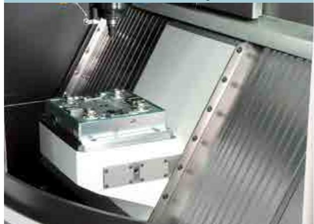
Mikron MILL S 400 with clamping chuck
