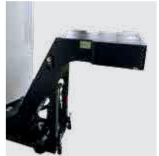
Chip conveyor to remove large volumes of chips
