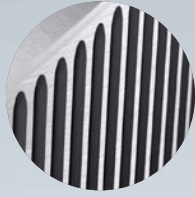
Laser engraving Surface finish reduced to Ra 1.0 \mu\text{m}
