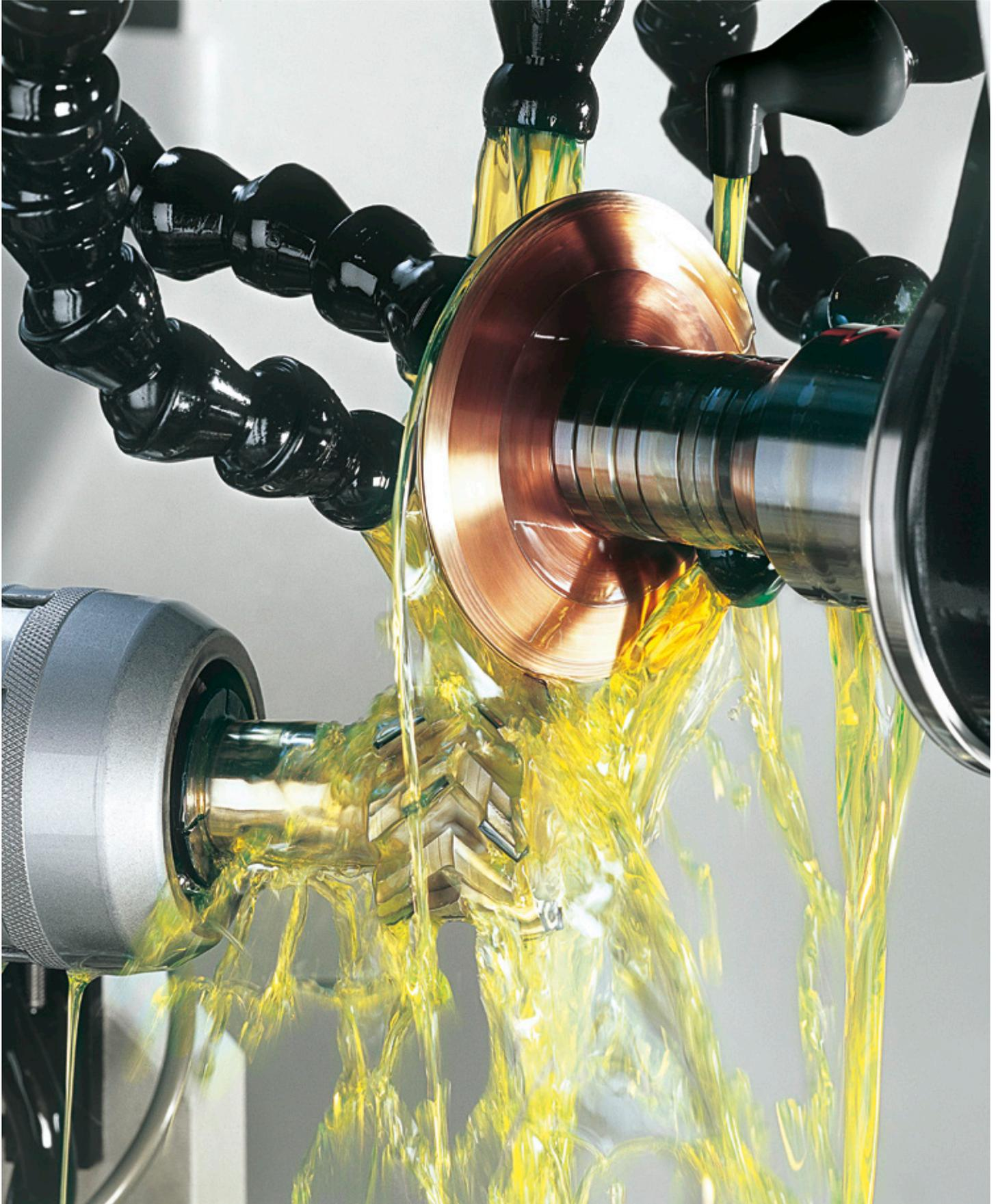
With the up to 3-stage rotary eroding procedure as standard, the HELITRONIC POWER DIAMOND sets new benchmarks for quality for PCD tools. The HELITRONIC POWER DIAMOND is an economic investment for both the production and resharping of PCD/CBN and HM/HSS tools in the diameter range of 3 to 320 (400) mm.
