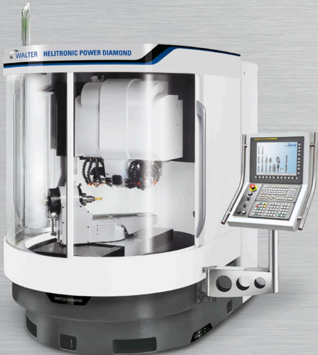
HELITRONIC POWER DIAMOND – the basic version with a belt-driven spindle and two ends.
