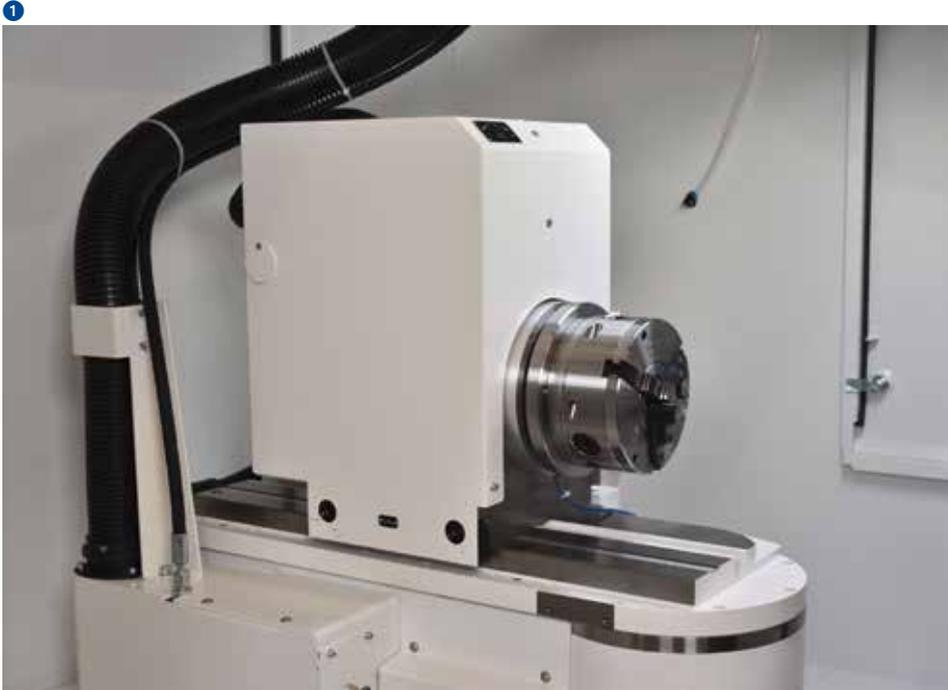
The high-precision workhead is equipped with special bearings and guarantees the highest roundness accuracy. The A4/MT5 spindle nose complies with the DIN/ISO 702-1 standard. The airlift simplifies adjustment when setting up or resetting the workhead. A high-precision C axis, with direct measuring system on the workhead spindle, is available for form and thread grinding.
