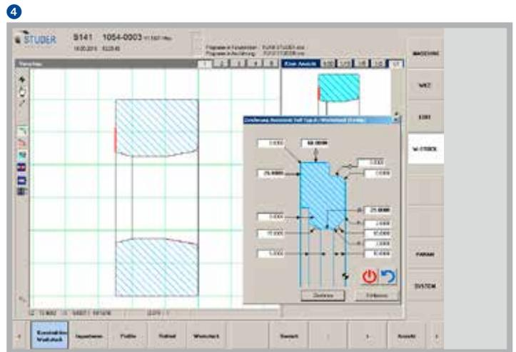
The machine control is equipped with the StuderSIM operating system. This operating system, specially developed for internal grinding applications, enables the programming of all basic cycles for grinding, dressing and process-supporting measurement. The basic cycles such as surface grinding, bore grinding, cone grinding, thread grinding, dressing and measurement are defined in the Parameter Input window.
