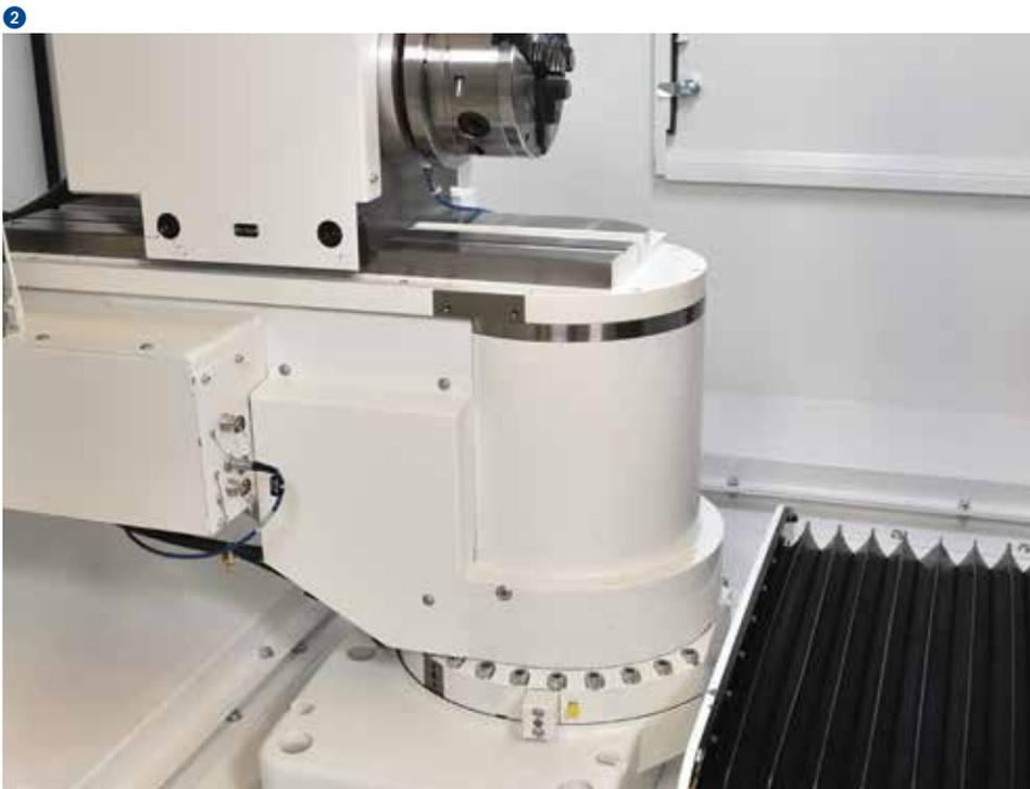
The automatic B-axis with a swiveling range of  $+61^{\circ}$  to  $-91^{\circ}$  has a direct drive, which enables very quick and precise positioning. This enables extremely precise grinding with interpolation of the B-axis to machine radii. The high-resolution direct measuring system guarantees a positioning range of the high-precision B-axis  $<1''$ .
