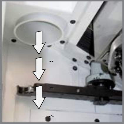
Supply air for dust extraction
