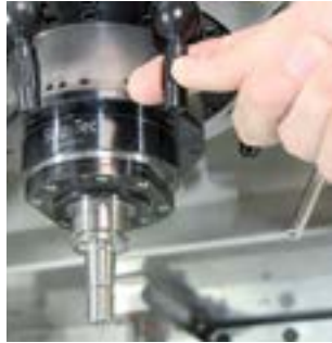
Spray ring with up to nine individually adjustable nozzles
