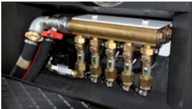
Five separate cooling circuits for the motors of the drives in the X, Y, Z, B/C axes, and the spindle motor.
