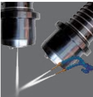
Air through spindle/spindle slots
