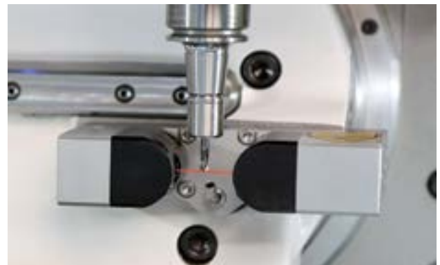
Precise measurement of very small tool diameters from 25 \mu m to 20 mm
