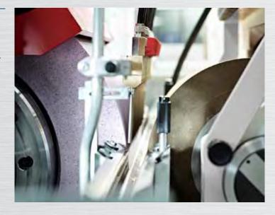
The KRONOS L centerless external cylindrical grinding machine is designed for infeed and throughfeed grinding in the diameter range of 5 to 250 mm and with a maximum infeed width up to 655 mm. The basis of the machine is a Granitan® bed, which guarantees the KRONOS L optimum damping characteristics and excellent thermal stability.
