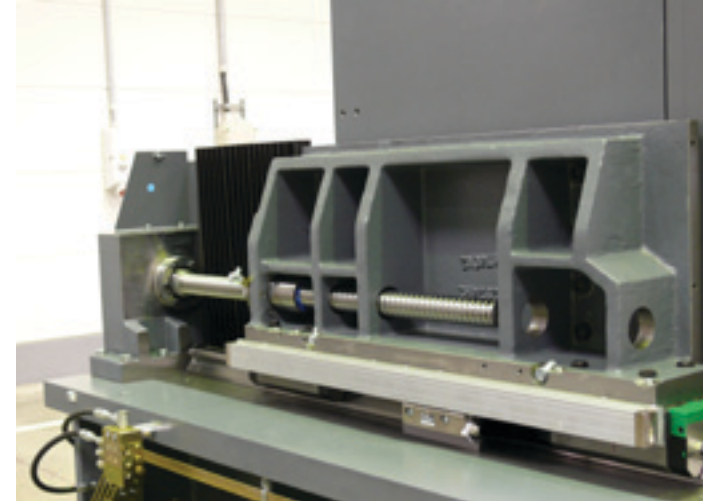
Z-axis with linear guideways, ground re-circulating ballscrews and linear glass measuring system
