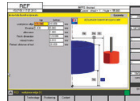
Parameter input screen for the external cylindrical grinding cycle
