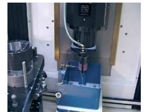
CNC dressing with single point diamond
