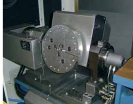
Double CNC indexing table for 5-axis continuous path controlled profile grinding
