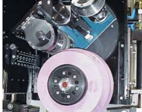
Double spindle CD-dressing system mounted on wheel head (E-axis)
