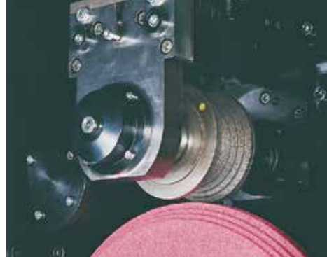
Single spindle CD-dressing system mounted on wheel hand (V-axis)
