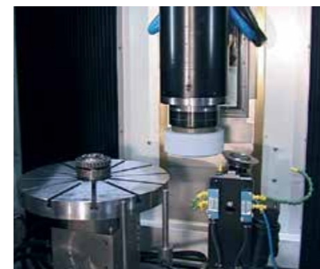
CNC dressing with rotary diamond disk
