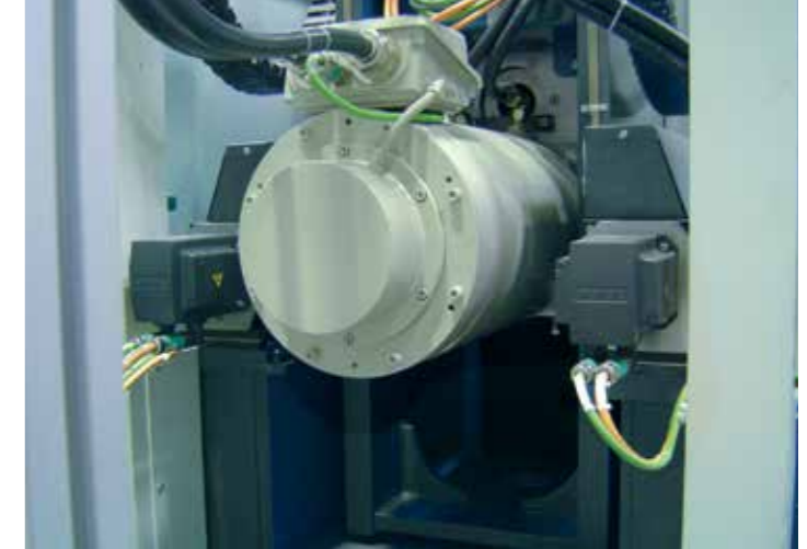
Z-axis with parallel drive system for increased rigidity (optional)
