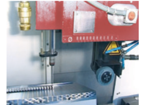
Measuring probe , pneumatically retracting from measuring position, up to 2 ½ axes, measuring accuracy +/- 1 µm
