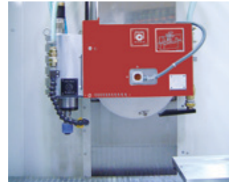
Vertical auxiliary grinding spindle for universal use in the mould and die industry with a power of up to 6 kW and up to 90,000 rpm
