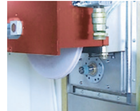
Horizontal auxiliary grinding spindle , automatically positioned in the working area, for the back-off grinding on broach tools using a min. wheel diameter of 30 mm
