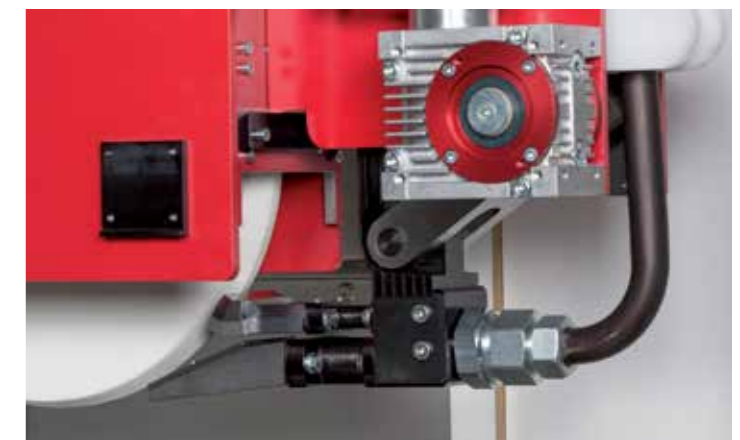
New way of grinding wheel cleaning, with newly developed nozzle positioner, 30% less grinding wheel wear, 30-40 bar nozzle pressure
