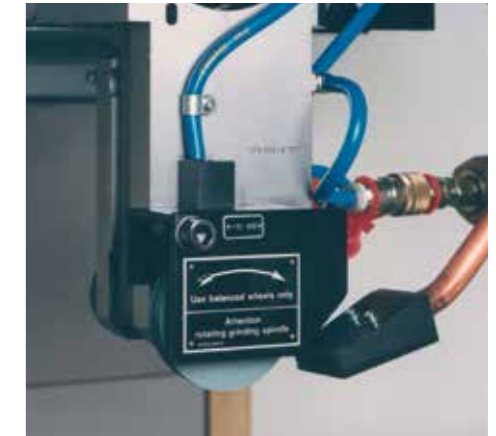
Horizontal internal grinding spindle , for grinding wheel diameters of 25 ... 70 mm, up to 45,000 rpm
