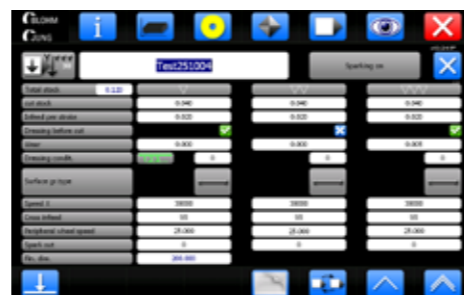
3 layer automatic grinding cycle: roughing, semi-finishing, finishing, spark-out with integrated dressing cycles. Only a few parameters are required to complete the cycle.
