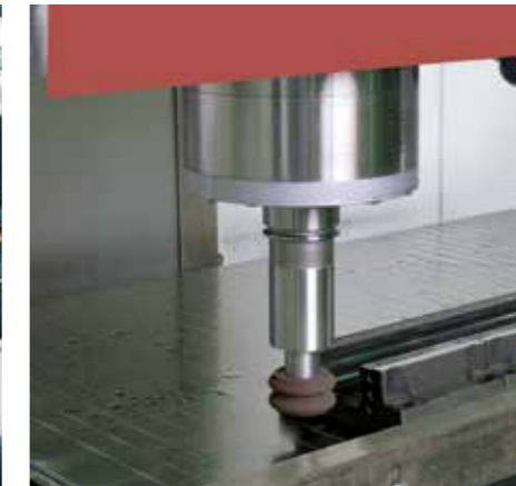
Vertical grinding spindle , on sliding bracket, 5 kW, max. 30,000 rpm
