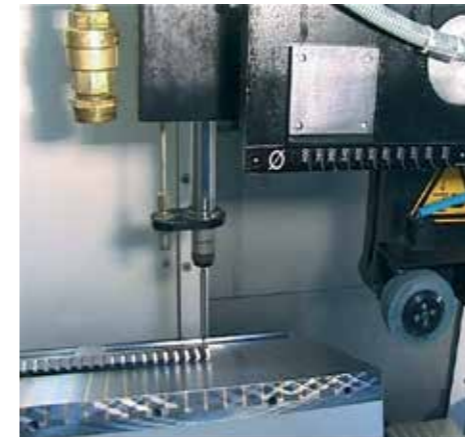
Measuring probe , pneumatically retracting from measuring position, measuring accuracy \pm 1 \mu\text{m}
