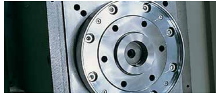
Cartridge type spindle with short taper for repeatable grinding wheel positioning
