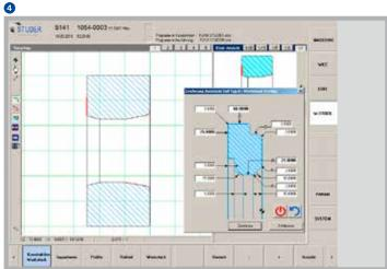
The machine control is equipped with the StuderSIM operating system. This operating system, specially developed for internal grinding applications, enables the programming of all basic cycles for grinding, dressing and process-supporting measurement. The basic cycles such as surface grinding, bore grinding, cone grinding, thread grinding, dressing and measurement are defined in the Parameter Input window.
