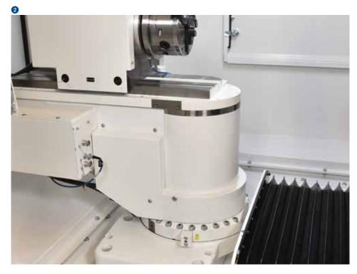
The automatic B-axis with a swiveling range of +61° to -91° has a direct drive, which enables very quick and precise positioning. This enables extremely precise grinding with interpolation of the B-axis to machine radii. The high-resolution direct measuring system guarantees a positioning range of the high-precision B-axis <1".
